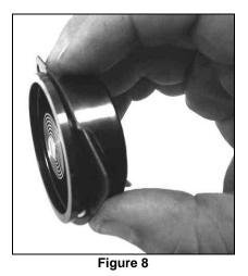
6. Install the new choke cap gasket onto the housing.
